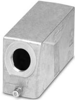
Sleeve housing B24, for single locking latch, material: Die-cast aluminum, salt water resistant, cable outlets: 1, lateral, 1x Pg21, height: 60 mm, cable gland: none, Standard
