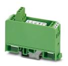
Relay module, with soldered-in miniature switching relay, contact (AgNi+Au): small to large loads, 2 changeover contacts, input voltage 230 V AC
