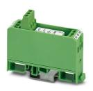
Relay module, with soldered-in miniature switching relay, contact (AgNi): medium to large loads, 2 changeover contacts, input voltage 230 V AC
