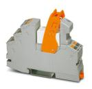
Pre-assembled relay module with Push-in connection, consisting of: relay base, power contact relay, plug-in display/interference suppression module, and retaining bracket. Contact type: 2 changeover contacts. Input voltage: 24 V DC
