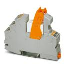
Preassembled relay module with Push-in connection, consisting of: relay base, multi-layer contact relay, plug-in display/interference suppression module, and retaining bracket. Contact switching type: 2 changeover contacts. Input voltage: 230 V AC
