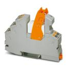
Pre-assembled relay module with Push-in connection, consisting of: relay base, power contact relay, plug-in display/interference suppression module, and retaining bracket. Contact type: 2 changeover contacts. Input voltage: 120 V AC
