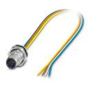
Device connector, rear mounting, PROFINET, 4-position, Flush-type male connector, straight, M12-SPEEDCON, coding: D , on free cable end, Rear mounting, Pg9, Individual wires, cable length: 0.1 m, 0.34 mm<sup>2</sup>, TPE litz wire, Alternative product in accordance with RoHS II without Exemption 6c (Pb <0.1%) item no.: 1239988
