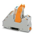
Pre-assembled relay modules with Push-in connection, consisting of: relay base, power contact relay, and retaining bracket. Contact type: 4 changeover contacts. Input voltage: 24 V DC
