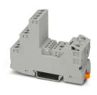
RIF-2... relay base, for industrial relay with 2 or 4 changeover contacts, screw connection, plug-in option for input/interference suppression modules, for mounting on NS 35/7,5
